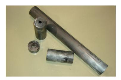
Lead window sash weights are becoming the choice by many contractors over steel cast weights due to the space savings obtained. Lead is approximately 40% smaller in size than steel and lead is non rusting material. Lead counterweights can also be easily cut on site if required and reused for other weights.
