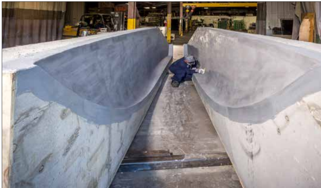
Preparing a large open mold, fabricated in Ceramicast tooling material, for a continuous lead pour. At 153,500 lbs (69,626 kg), the largest keel the company has cast to date was for the Bruce King-designed and Hodgdon-built 155' (47.2m) Scheherazade.
