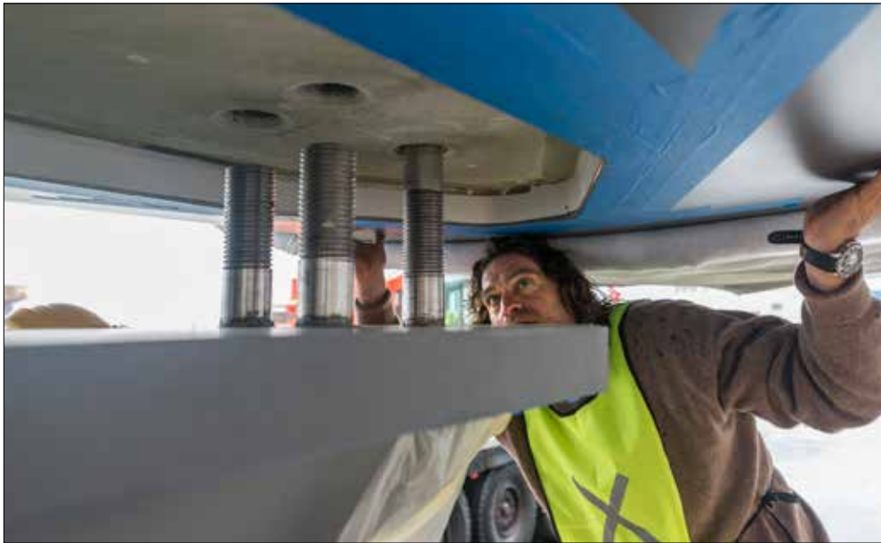
Precision and care are required in lowering Lady G's hull onto its 38,500-lb (17,463-kg) keel.
