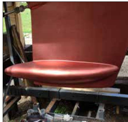
Left —The company offers a draft-reduction service that advises how much this deep-draft iron keel is to be shortened to allow the boat's access to shallower water.
